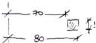
$$V_5 = \pi \times 10 (80^2 - 70^2) = \pi \times 10 \times 1900$$
