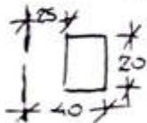
$$V_2 = \pi \times 20 (40^2 - 25^2) = \pi \times 20 \times 975 = \pi \times 10 \times 1950$$
