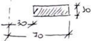
$$V_4 = \pi \times 10 (70^2 - 30^2) = \pi \times 10 \times 4000$$
