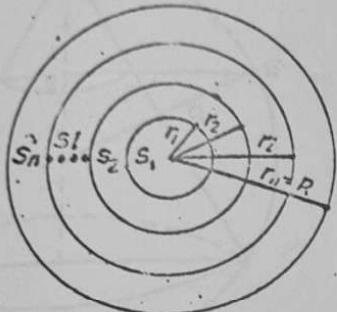
$$\therefore s_2 = s_1 = \frac{St}{n} \quad \therefore \pi(r_2^2 - r_1^2) = \frac{\pi R^2}{n}$$
